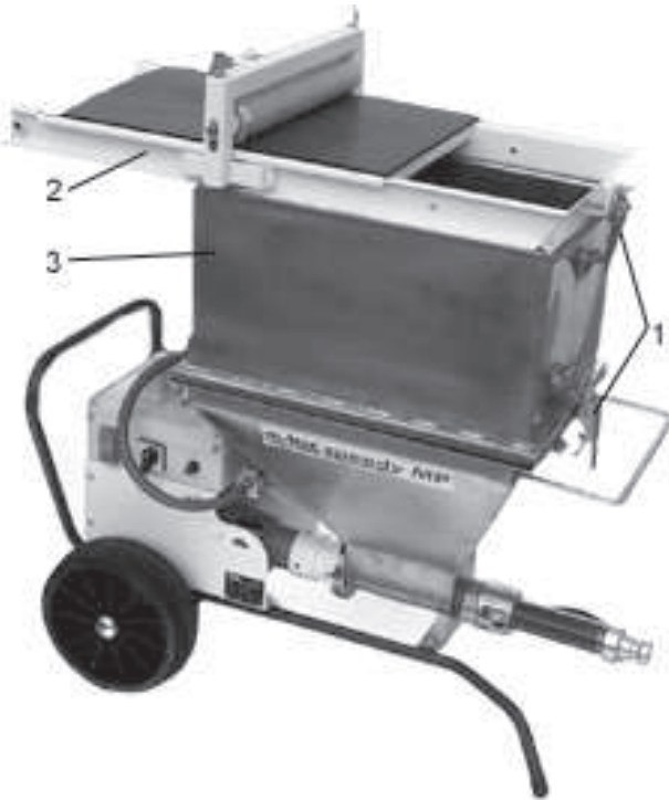
Fig. 8: Filling funnel and sack mangle installed
