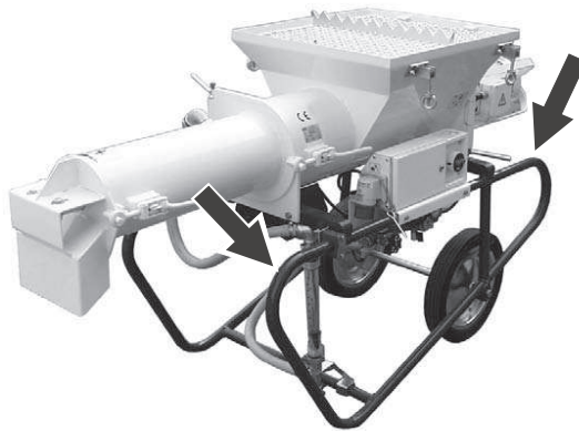
Fig. 6: Lifting points on the D30
