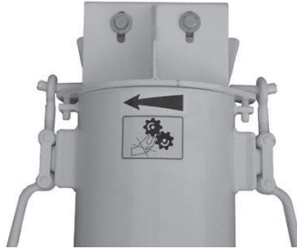
Fig. 9: Direction arrow on mixing tube
