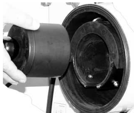
Fig. 26: Close feed unit with plug
