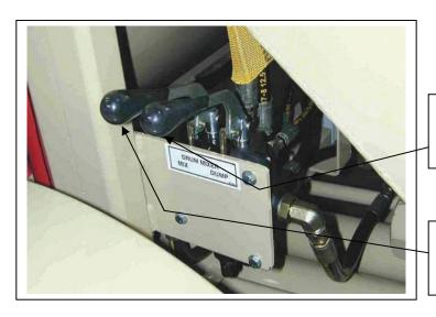
Mixer lift valve. Pull up to lift the mixer. Push down to lower the mixer.
