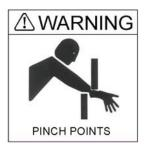
The mechanical linkage located on the side of the mixer, opposite the dump control valve, positions the mixer grate when the mixer is dumped. Because of the relative motion of this link, the mixer drum and the hopper produces a scissors movement which can pinch anything in its path. Confirm that this area is clear of all personnel when operating the mixer. Severe bodily injury can occur to any body member pinched.
