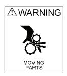
Never put hands in the lubricating wash box when the pump is operating. Oscillating linkage can amputate the fingers or hand. Severe injury can result. Never work on any part of the pump that is in motion while the motor is running. Take time to stop the motor and turn off/disconnect power supply.
