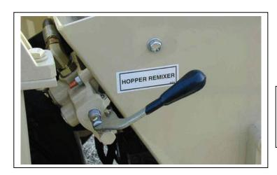
Re-mixer control valve. Push in for forward operation. Pull out for reverse operation. (Re-mixer optional on MR450)
