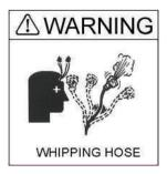
If the delivery system is blocked for any reason, or the line kinked at the start-up or during the pump operation, the pump pressure could straighten out the kink or force out the blockage. The rapid surge of material could cause the line to whip or move in such a manner that it may cause injury to personnel.
