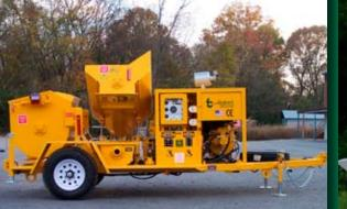
Hydraulic receiving hopper lift for easy clean-out
