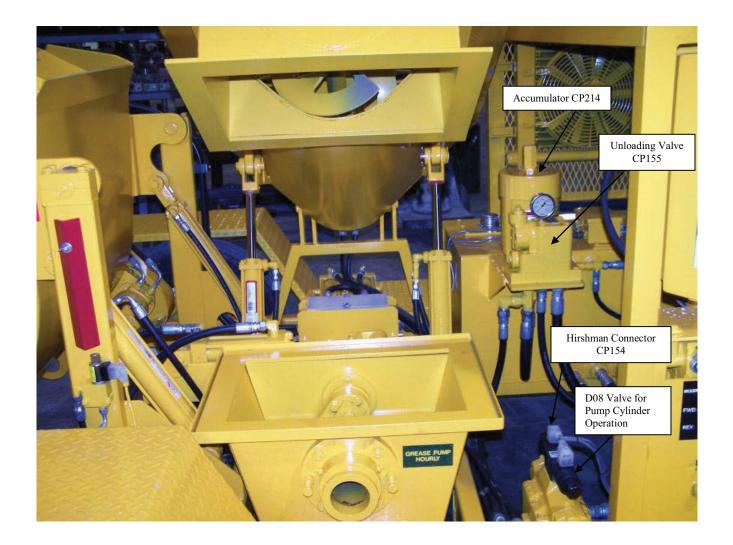
~If it is necessary to remove a hydraulic hose, be sure to keep fittings and hoses closed using plastic plugs or tape. If hoses are replaced, be sure the replacement hose has been flushed out and is clean. REMEMBER, BY KEEPING YOUR HYDRAULIC FLUID CLEAN, YOU CAN REDUCE POTENTIAL HYDRAULIC PROBLEMS BY 92%.
