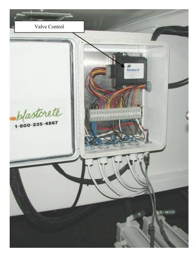
The switch controlling the forward and reverse function informs the "Valve Control" which side of the coil on the swing tube valve to activate. There is no change to the pumping cylinder to accomplish this task. This allows the machine to either pump material out the hose or draw material back through the hose.
