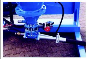
^View at discharge armature at the pressure vessel UELZENER T115 and hose connection.
