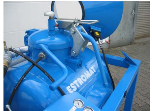
Safety lock for dome
