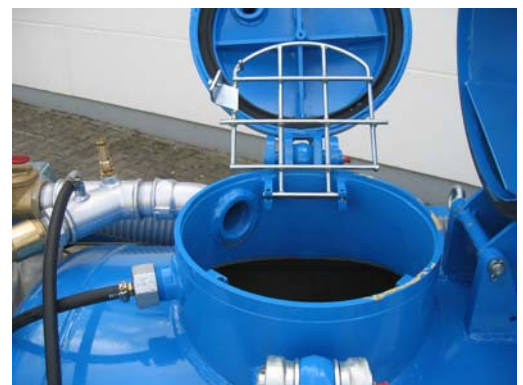
Safety screen in the vessel dome
