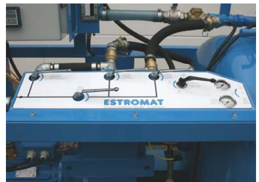
Compressed air control armatures
